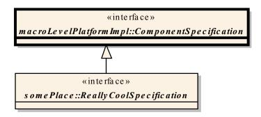
Functionality of a component can be extended without breaking the code of existing users of the component
